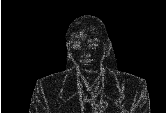
Fig.4. Absolute difference between the original object 'Akiyo' and the watermarked one, magnified by a factor 32.
